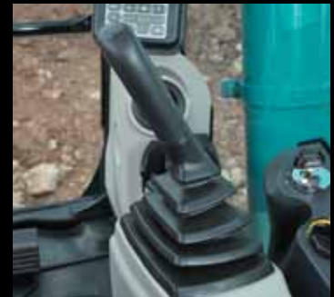
Double slides allow adjustment for optimum comfort
